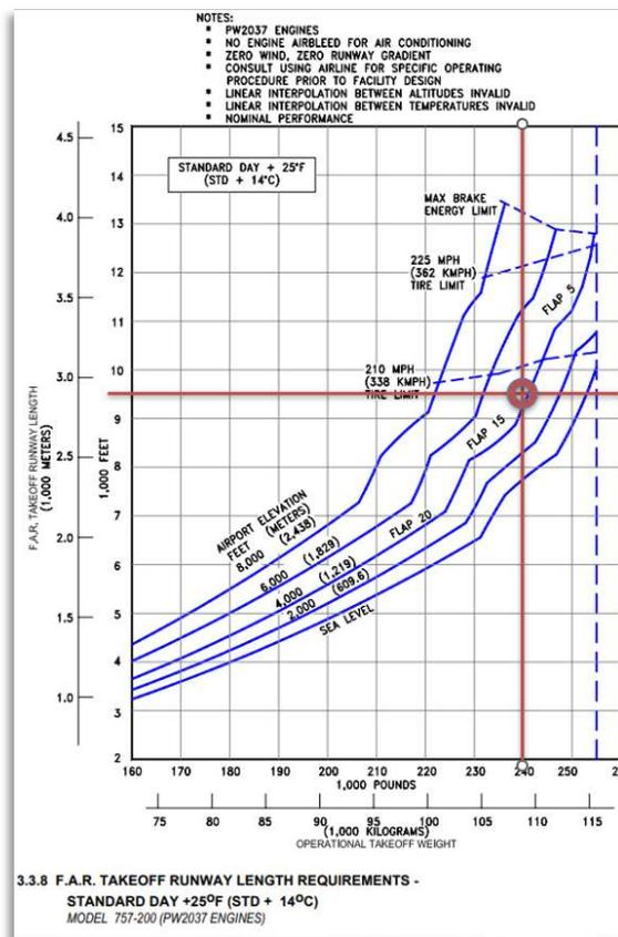
At top-right is a runway length table for airport design issued by Boeing for the 757-200 aircraft. This type of table is used by airport planners to design runways. For example, this table indicates that on a hot day (84 degrees Fahrenheit) at an airport with an elevation similar to DNA at approximately 4,000-feet above sea level and a runway length of approximately 9,500-feet, a B757-200 could takeoff at approximately 95 percent of its
